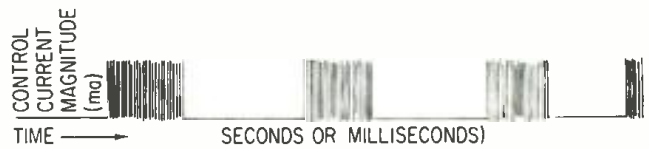
Figure 4. The wave-form of pulse bursts, useful for testing audio equipment and other experimental applications including electronic music.
